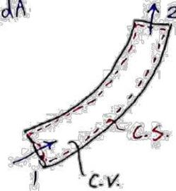
$$\Rightarrow \dot{Q}_{c.v.} = \int_{A_1} (e_1 + \frac{p_1}{\rho_1}) \rho \vec{V}_1 \cdot d\vec{A}_1 + \int_{A_2} (e_2 + \frac{p_2}{\rho_2}) \rho \vec{V}_2 \cdot d\vec{A}_2$$
