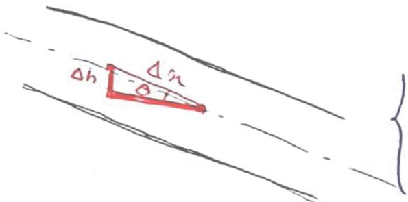
$$\left. \begin{array}{l} \sin\theta = \frac{\Delta h}{\Delta n} = \frac{\partial h}{\partial n} = \frac{dh}{dn} \\ h = n \sin\theta \end{array} \right\}$$
